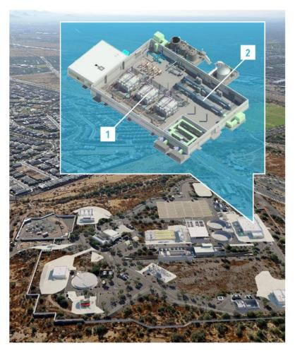
Above is a rendering of the future upgraded Cave Creek Water Reclamation Plant, including a rendering of the facility that will purify recycled water to drinking water using (1) Reverse Osmosis and (2) UV Advanced Oxidation technologies. This is how Advanced Water Purification works.
