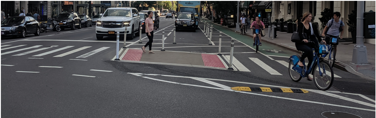
Parked cars serve as a barrier between bicyclists and the vehicle lane. Barriers could also include flexible posts, bollards, planters, or other design elements.
