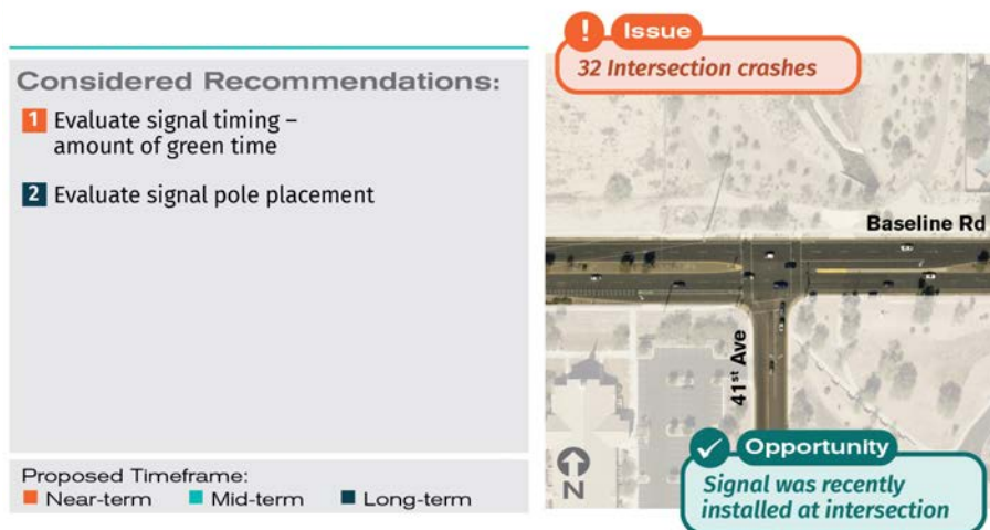
Figure 5.18 41 st Ave / Baseline Rd: Recommended Safety Improvements
