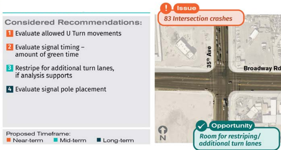
Figure 5.39 35 th Ave / Broadway Rd: Recommended Safety Improvements:
