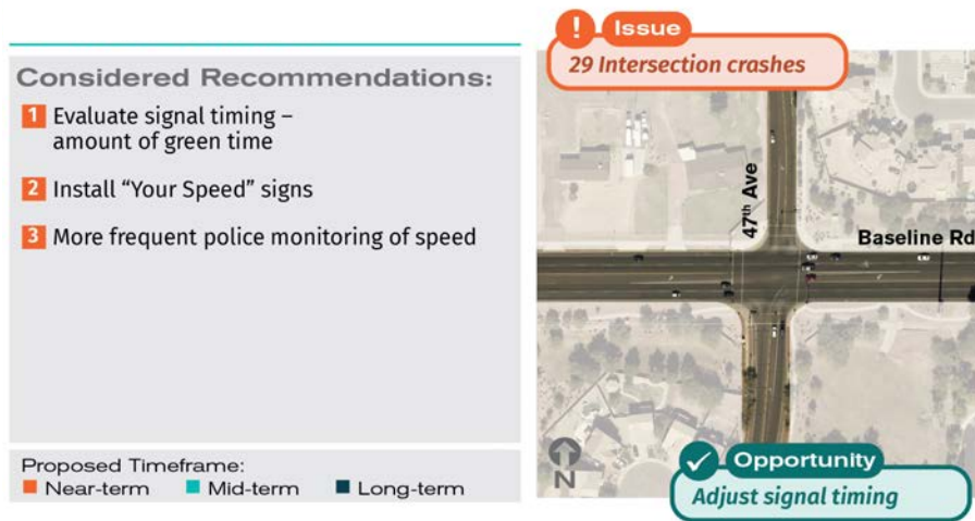
Figure 5.16 47 th Ave / Baseline Rd: Recommended Safety Improvements
