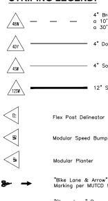
4" Broken White Line with a 10' Line Segment and a 30' Gap
