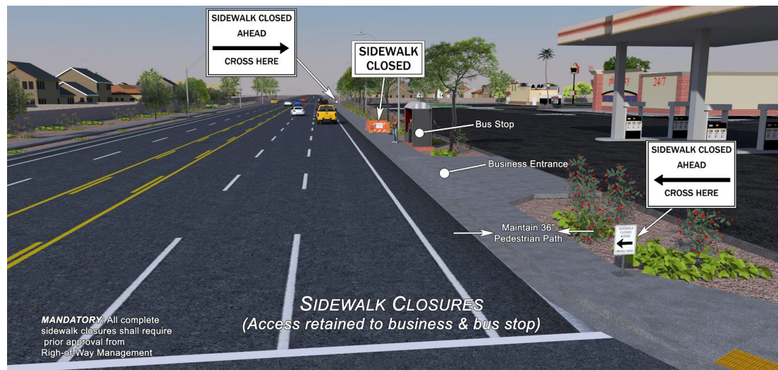
Figure 7 – Sidewalk Closure Midblock (Access Retained to Business/Bus Stop)
