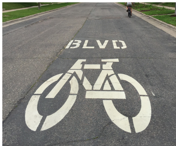
An example of an large pavement marking to reinforce that the street is a Bike Boulevard.
