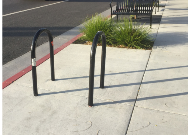
Inverted-U racks provide two points of contact.
