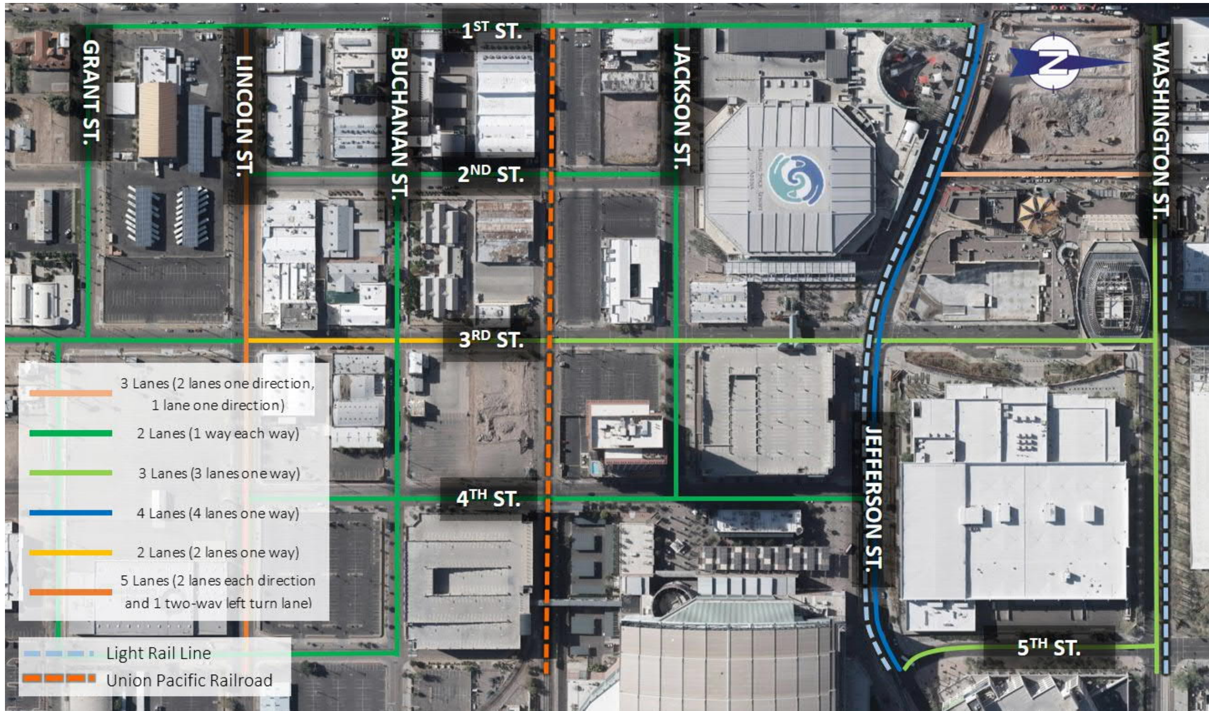
Figure 2: Study Area Roadway Cross-Sections
