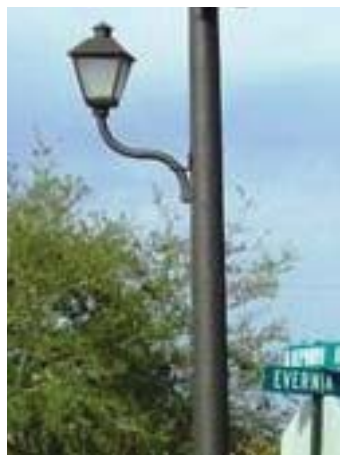
Photo: Standard APS Colonial Salem Light Fixture for Pedestrian Lighting
