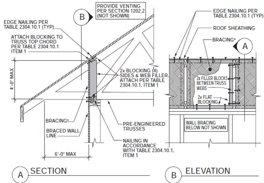
a. Methods of bracing shall be as described in Table 2308.6.3(1) DWB, WSP, SFB, GB, PBS, PCP or HPS.
