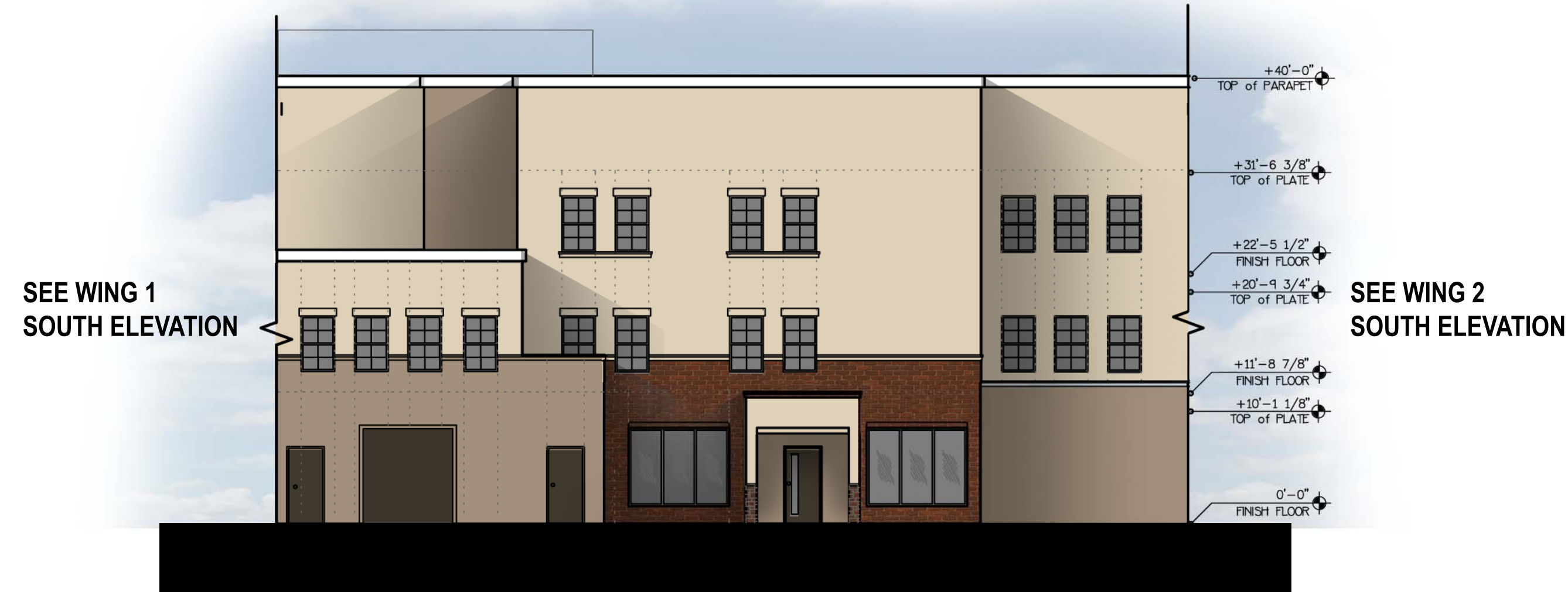
COMMON AREA SOUTH ELEVATION SCALE: 1/10"=1'-0"
