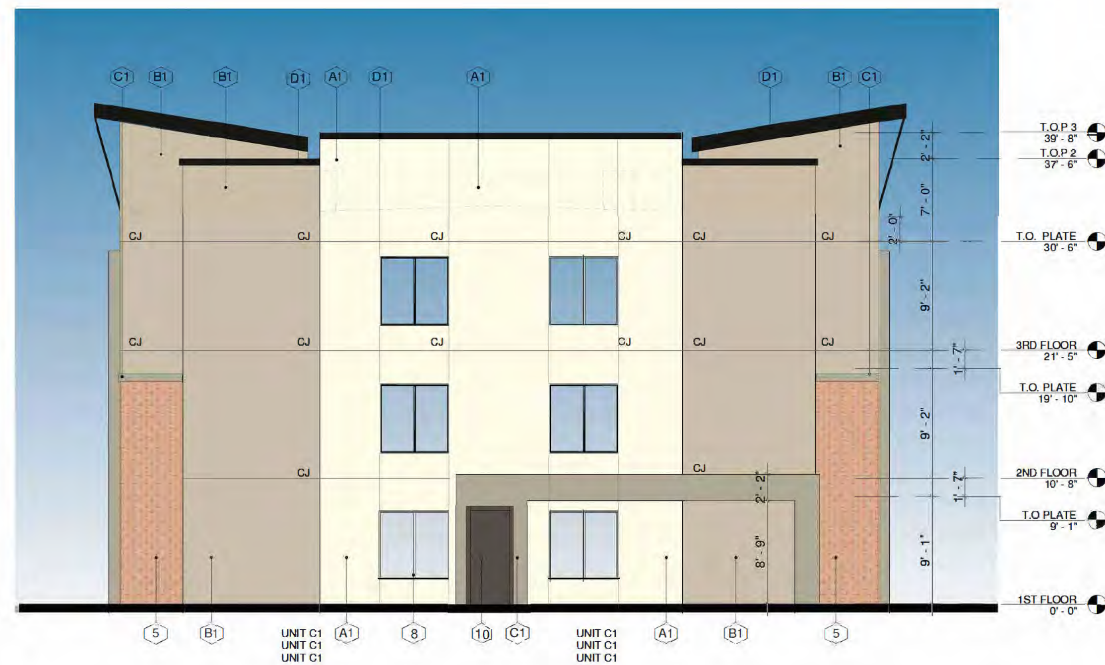
RIGHT / LEFT ELEVATION - BUILDING TYPE 1 1/8" = 1'-0"
