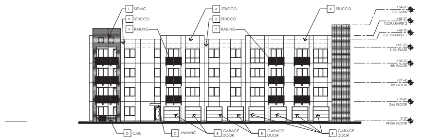
2 BUILDING 4 - NORTH ELEVATION SCALE: 1/16" = 1'-0"
