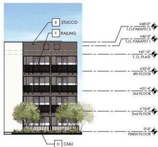
7 BUILDING 3 - SOUTHWEST ELEVATION SCALE: 1/16" = 1'-0"
