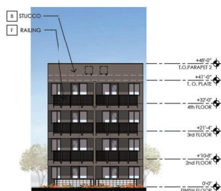
1 BUILDING 2 - SOUTHWEST ELEVATION SCALE: 1/16" = 1'-0"
