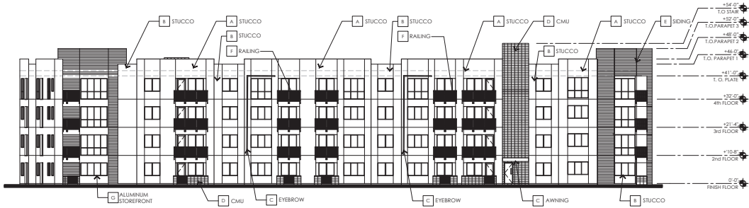
2 BUILDING 3 - NORTH ELEVATION SCALE: 1/16" = 1'-0"
