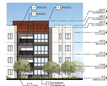
3 BUILDING 3 - NORTHEAST ELEVATION SCALE: 1/16" = 1'-0"
