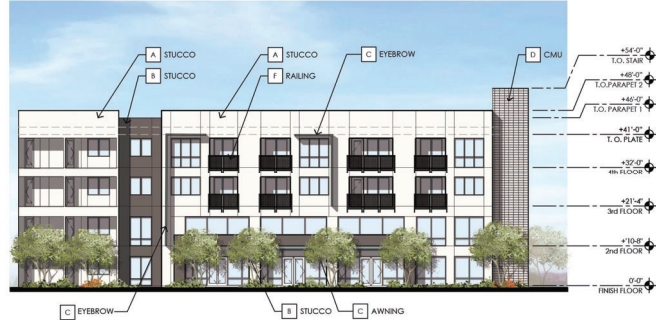
2 BUILDING 4 - SOUTH ELEVATION SCALE: 1/16" = 1'-0"
