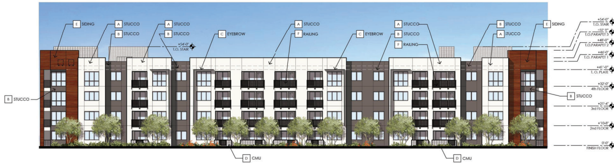
3 BUILDING 4 - EAST ELEVATION SCALE: 1/16" = 1'-0"
