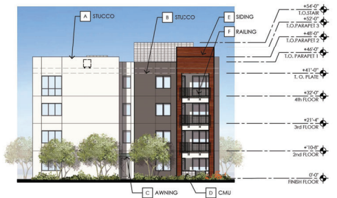
5 BUILDING 3 - SOUTH ELEVATION SCALE: 1/16" = 1'-0"
