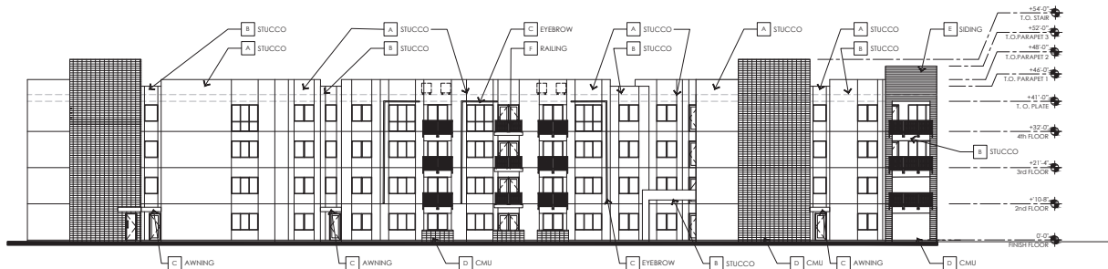
1 BUILDING 4 - WEST ELEVATION SCALE: 1/16" = 1'-0"
