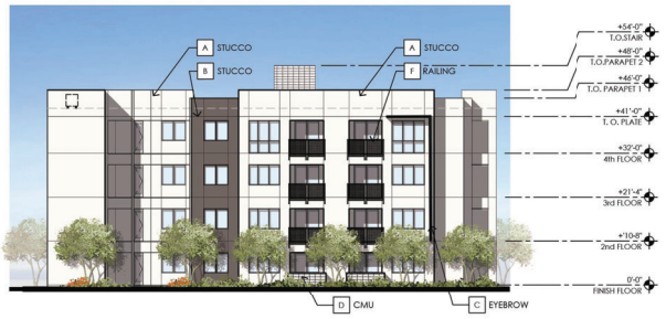
6 BUILDING 3 - WEST ELEVATION SCALE: 1/16" = 1'-0"
