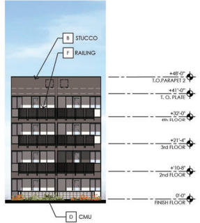
3 BUILDING 4 - NORTHEAST ELEVATION SCALE: 1/16" = 1'-0"
