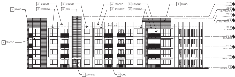
3 BUILDING 2 - EAST ELEVATION SCALE: 1/16" = 1'-0"
