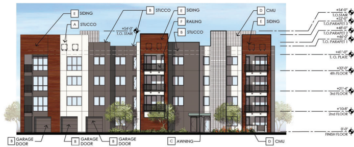
4 BUILDING 6 - SOUTH ELEVATION
