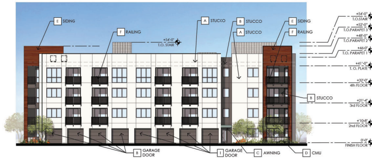
1 BUILDING 5 - SOUTH ELEVATION
