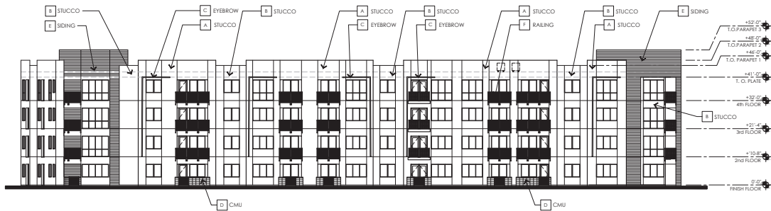
1 BUILDING 2 - NORTH ELEVATION SCALE: 1/16" = 1'-0"
