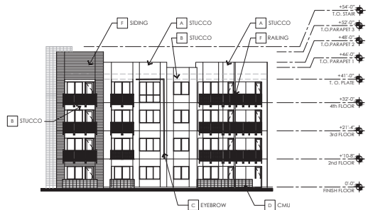
5 BUILDING 4 - NORTH ELEVATION SCALE: 1/16" = 1'-0"
