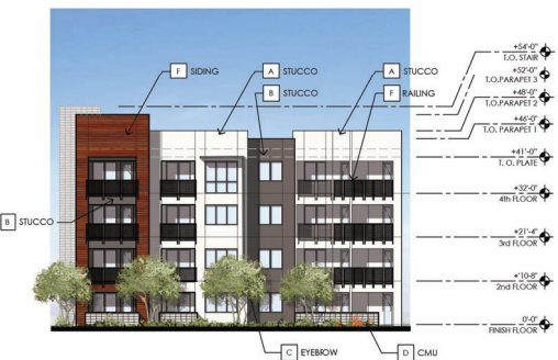
5 BUILDING 4 - NORTH ELEVATION SCALE: 1/16" = 1'-0"
