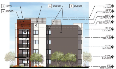
3 BUILDING 2 - WEST ELEVATION SCALE: 1/16" = 1'-0"
