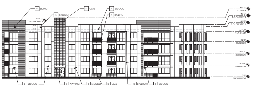
4 BUILDING 3 - EAST ELEVATION SCALE: 1/16" = 1'-0"
