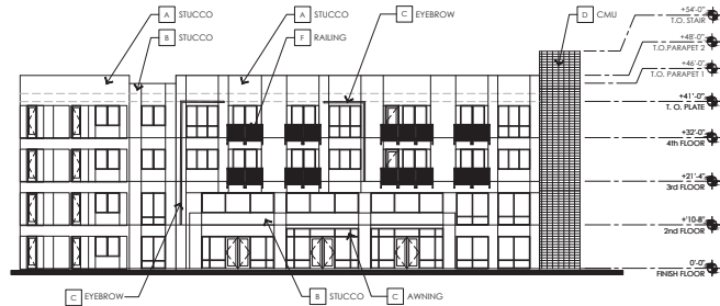
2 BUILDING 4 - SOUTH ELEVATION SCALE: 1/16" = 1'-0"
