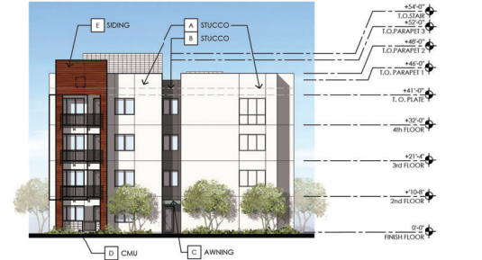
1 BUILDING 3 - WEST ELEVATION SCALE: 1/16" = 1'-0"
