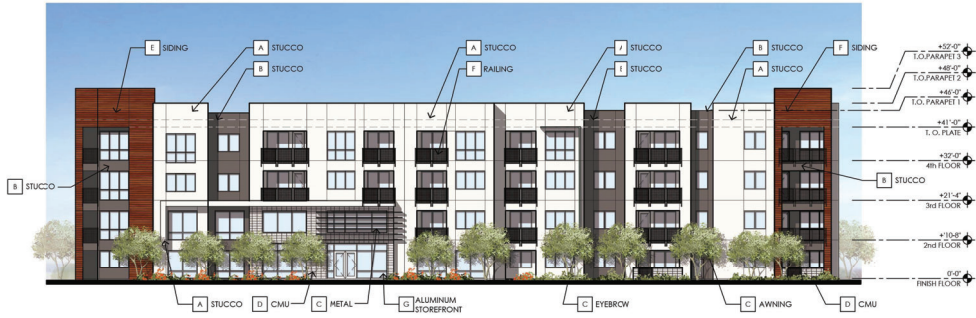
1 BUILDING 4 - SOUTH ELEVATION SCALE: 1/16" = 1'-0"
