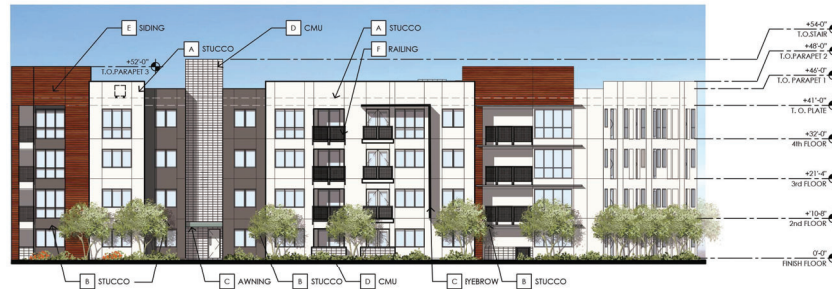
4 BUILDING 3 - EAST ELEVATION SCALE: 1/16" = 1'-0"
