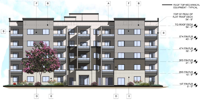
BUILDING TYPE 2 - FRONT ELEVATION
