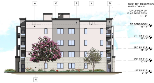
BUILDING TYPE 1 - RIGHT ELEVATION
