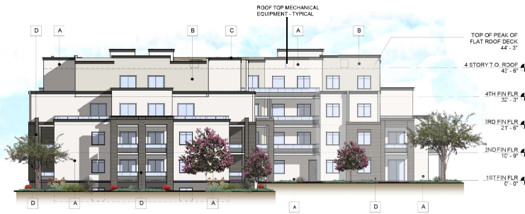
BUILDING TYPE 3 - RIGHT SIDE ELEVATION 1/16" = 1'-0"
