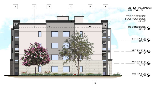
BUILDING TYPE 1 - LEFT ELEVATION
