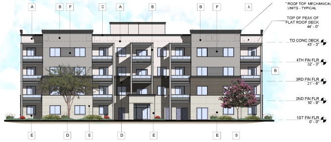
BUILDING TYPE 1 - FRONT ELEVATION
