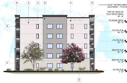
BUILDING TYPE 2 - RIGHT ELEVATION
