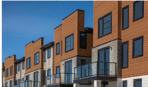
5.2b.7 When materials turn the corner from a primary frontage, the materials and detailing should be consistent with the primary facade for a minimum distance of 30 feet along the secondary or rear frontage.
