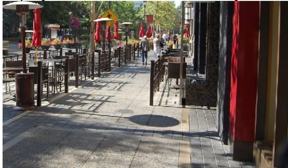
4.2b.4 Sidewalks should be designed to allow visibility around sharp corners. Avoid tall fences, inset corners, and overgrown vegetation at corners to maintain visibility and safety. 4.2b.5 Wider sidewalks may have different types of paving to denote different zones for amenities and pedestrian activity.
