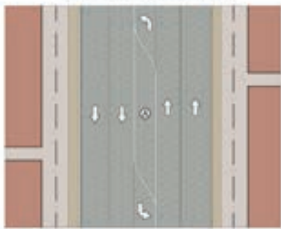
A. Existing 2-lane with turn lane
