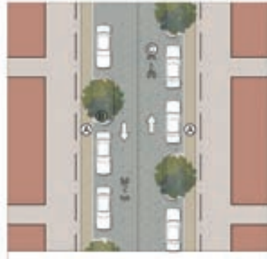
A. Add min. 5' sidewalk where missing B. Add tree pockets C. Add shrubs
