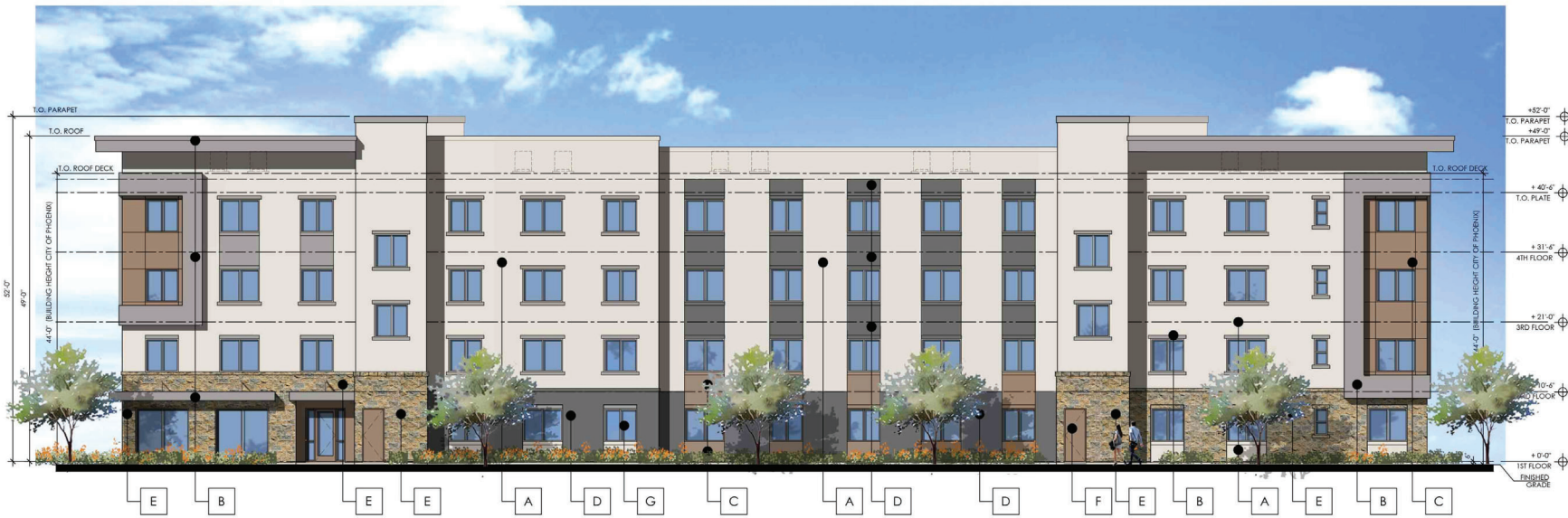
EAST ELEVATION SCALE 1/8" = 1'-0"
