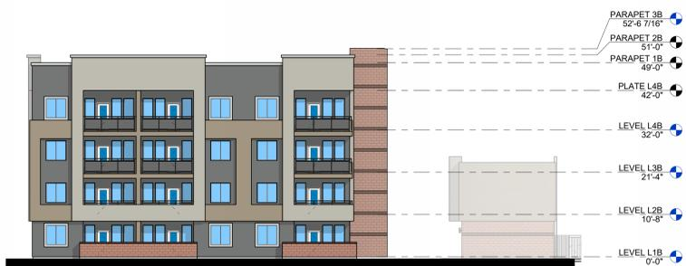
7 BLDG 2&3 - WEST ELEVATION SCALE: 1/16" = 1'-0"
