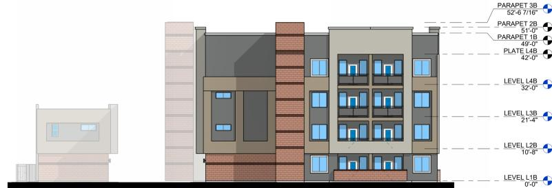
5 BLDG 2&3 - EAST ELEVATION SCALE: 1/16" = 1'-0"
