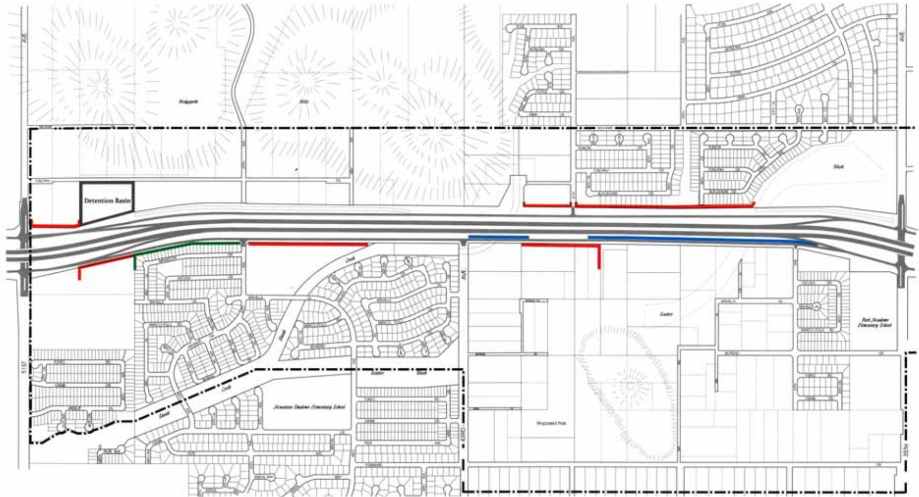
Figure 27 PROPOSED NOISE WALLS Outer Loop Freeway - Loop 101 Segment 1: 51st Avenue to 35th Avenue
