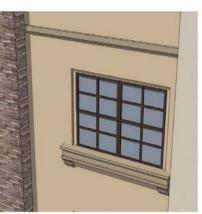
WINDOW TRIMS WITH STONE BASE; STONE TRIMS TO BREAK UP THE WALL SURFACES
