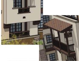
DECORATIVE BALCONY ELEMENTS WITH RAFTER BASE TAIL PROFILES & BRICK OR IRON METAL RAILING
