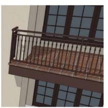
BALCONY TYPE - 1 (ROOFED BALCONY WITH IRON RAILING)
