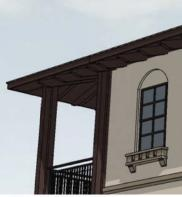
TERRA COTTA TILE ROOFING (3:12 PITCHED & 4'-0" HT.) & TRIM PROFILE; EAVE OVERHANG WITH EXPOSED RAFTER TAILS
