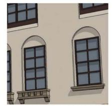
ARCH ABOVE DOOR OR WINDOW WITH STONE BASE WITH DIFFERENT PROFILES OR RECESSED ANGLE BASE
