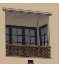
BALCONY TYPE - 2 (ROOFED BALCONY WITH TILE RAILING WITH 6"TRIM ABOVE RAILING)
