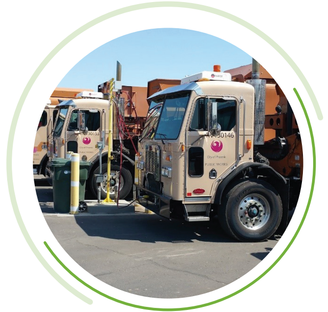
Solid Waste Garbage Trucks being slow-filled with compressed natural gas.
