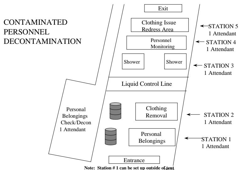
NOTE: Optimally, the Technical Decontamination Setup will be operated by 5 technicians
