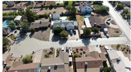
Cool pavement coating reflects a higher portion of the sunlight that hits it, hence absorbing less heat. Because of this higher reflection, the coating has the potential to offset rising nighttime temperatures in the region.
