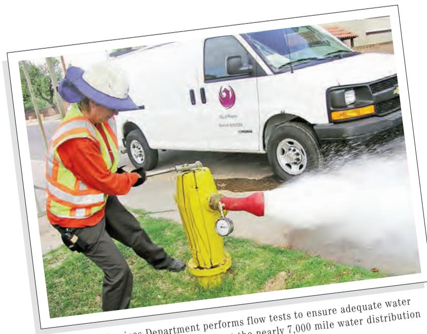
The Water Services Department performs flow tests to ensure adequate water pressure for fire protection throughout the nearly 7,000 mile water distribution system.
